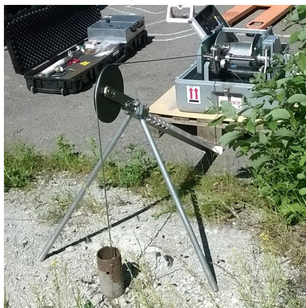
The Wassara Explorer™ being used to survey a near-vertical hole in a winch and wireline configuration.
