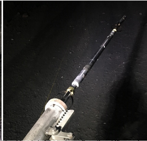
The Wassara Explorer™ (battery version) in a blast-hole fan survey configuration at Kiruna mine.
