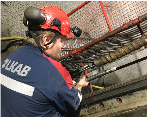
The Wassara Explorer™ about to be pumped down for an OUT-run survey of an exploration hole in the Kiruna mine.
