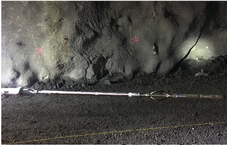
The Wassara Explorer™ (battery version) in a blast-hole fan survey configuration at Kiruna mine.
